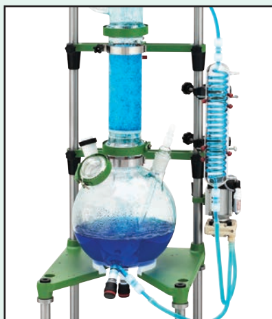
Gas scrubber systems neutralize corrosive gas and vapors.
